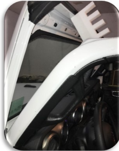
Fig. 2 Windshield Propped Forward
