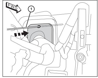
13. Secure the end of the hood switch harness to the fish wire with tape. Pull the end of hood switch harness (B) through to the inside driver footwell. Apply RTV sealant to the hood switch wiring convolute and pull the wiring into the nipple to seal the wiring at the nipple.
