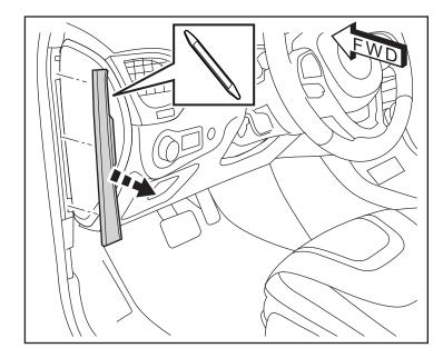
10. Carefully pry off the trim panel at the end of the dashboard on the driver side. Remove two (2) screws and two (2) clips from lower trim panel. Pry off the lower trim panel under the steering column. Pull the hood switch harness (B) through to the inside footwell.
