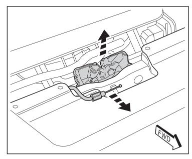
4. Reconnect the hood latch release cable to the back of new hood latch assembly. Position the new hood latch (A) with the alignment marks and secure with two (2) hex bolts. Tighten bolts to 9 Nm (80 in. lbs.)
