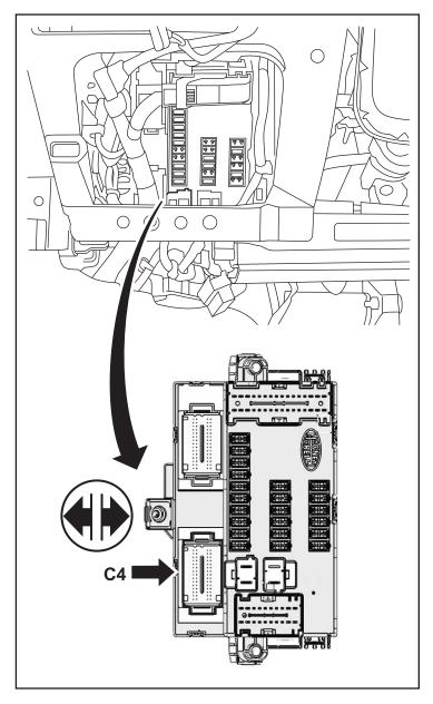
15. Press in on the release tabs at the back of the connector and slide the plug out from the outer casing.
