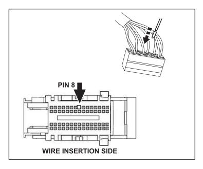
18. Reinstall the outer casing on the connector. Plug all connectors back into the BCM.
