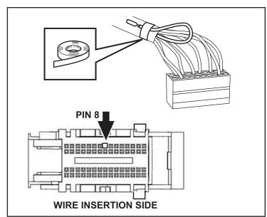
17. Insert the tab wire connector from hood switch harness (B) into Pin 8 on the connector.
