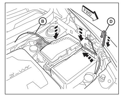
8. At the fender edge next to the battery, remove the existing ground wire hex nut. Position the ground ring terminal from the main harness (B) and reattach the nut to secure.
