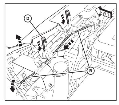
7. Route the hood switch harness (B) along the existing vehicle harnesses on the driver side and back towards the rear of the engine compartment.
