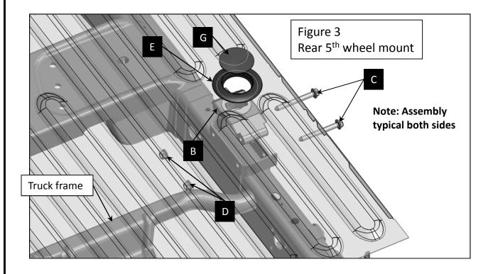
Note: check hitch frequently, making sure all fasteners and ball are properly tightened. A hitch or ball which has been damaged should be removed and replaced. Observe safety precautions when working beneath a vehicle and wear eye protection. Do not cut access or attachment holes with a torch.
