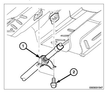
6. Remove and discard the driveshaft to differential flange bolts (1) and washers (2).
