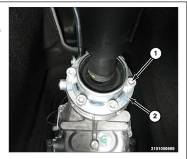
4. Position the center bearing (1) in place and loosely install the center bearing to body bolts (2) by hand. **Do not tighten at this time**.
