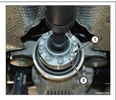
7. With the aid of an assistant, remove the driveshaft assembly.
