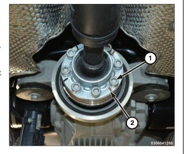
Install driveshaft into position at the transmission flange. Install the NEW driveshaft to transmission flange washers
