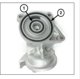
Install the Oil Filter Adapter to the engine block using the three bolts and tighten to 12 N·m, (9 ft·lbs).
