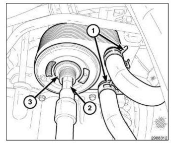
Insert the rubber outer oil seal (2) in the grove on the oil filter adapter.
