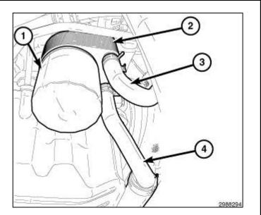
Remove the clamps (1) from the cooling hoses at the oil cooler and remove hoses if connected.
